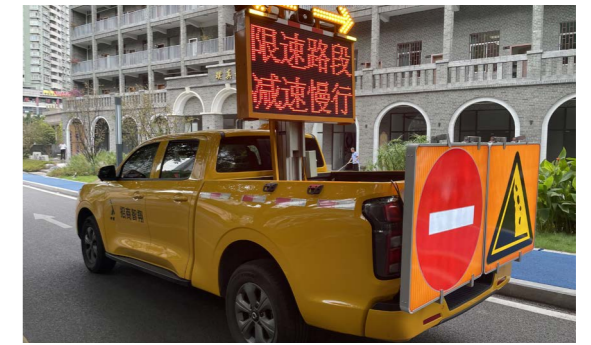
Vehicle-mounted mobile signs-transparent panel display self-luminous signs
